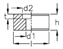
$$\begin{array}{lll} b & = 12 \\ d1 & = 6 \\ d2 & = 10 \\ H & = 8 \\ L & = 20 \\ screw = M5x12 \end{array}$$
